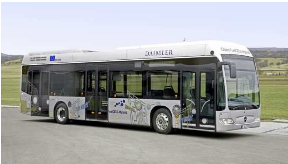
Figure 4 – Le CITARO Fuel Cell Hybrid Bus (2009)
